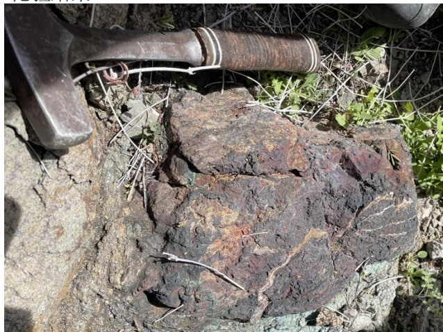
Cu-bearing magnetite skarn in quartz diorite dike 石英闪长玢岩脉中的含铜磁铁矿矽卡岩
